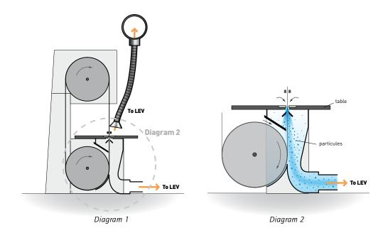
To improve capture of the dust, the table block (the piece around the saw at work table level) should be modified by drilling as shown in the diagram below.
